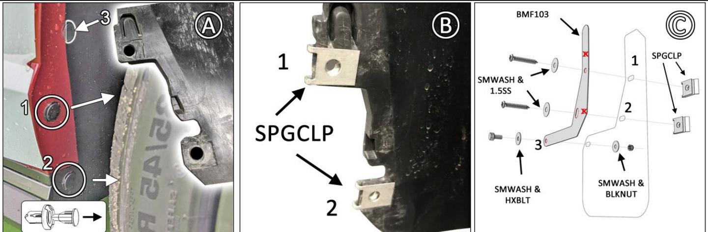
**REAR MUD FLAP** Do not fully tighten fasteners until mud flap is completely aligned to vehicle.
