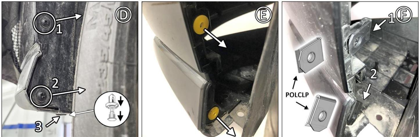
**FIGURE G** Reinstall factory fastener 3. Wipe area clean before adhering SMF113-LR/RR against mounting points.
